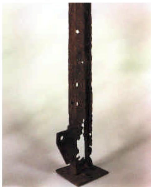
**Figure 11** Corroded steel stanchion
