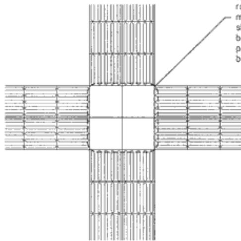
Orientation of slabs in the shared area should be dictated by the most heavily trafficked route. The tactile paving on the more lightly trafficked route should be installed so that the bars run transversely across the pedestrian travel for 1200mm before the shared area.
